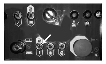
Figure 11.2 - Diesel/Electric Selection Switch
