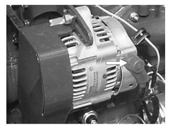
Figure 5.3 - Alternator Output Shutdown
