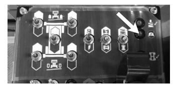
Figure 2.4 - Platform Overload Light
