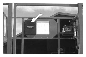
**Figure 7.34 - Operator Manual Holder** Check that the operation manual is in the holder.
