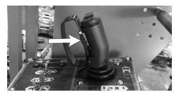
Figure 2.8 - Joystick Safety Control
