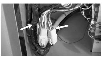
Figure 7.10 - Wiring Harnesses and Connectors
