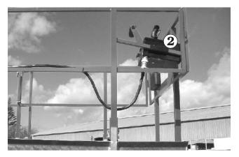
Figure 6.1.2 - Control Box Location, Platform Position
