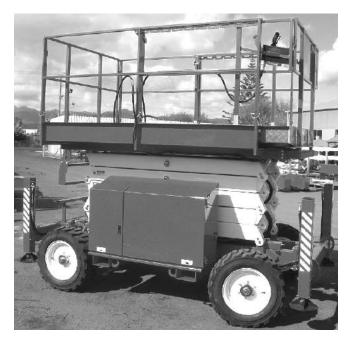
Figure 10.1 - Correct Stowed Position
