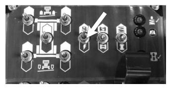
Figure 11.4 - Fuel Switch, Platform
