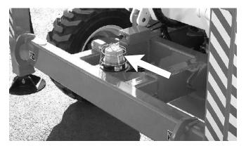
Figure 7.27 - Flashing Light
