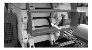
Figure 7.11 - Wiring Harness in the Scissor Stack
