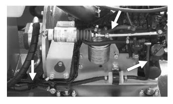
Figure 7.5 - Fuel Leaks in Hoses & Joints
