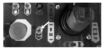
Figure 2.10 - Operator Horn
