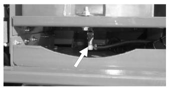
Figure 7.4 - Fuel Leaks at Tank
