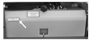
Figure 4.4 - Hydraulic Oil Level
