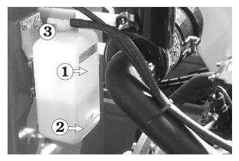
Figure 7.7 - Engine Coolant Level
