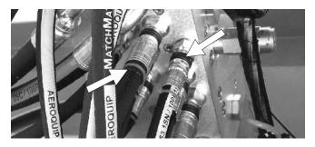
Figure 7.14 - Check Fittings at Valve
